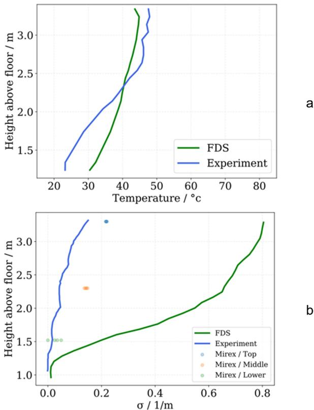
Fig. 6. Simulation results for the temperature development (a) and light extinction coefficient (b) at  $t = 300$  s as a function of height.
