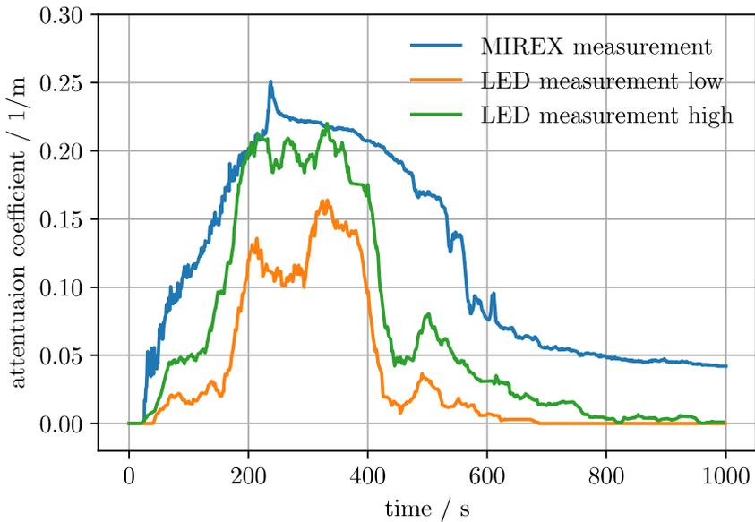
Fig. 2. Comparison of a MIREX measurement with the results of the LED-measurements. The data based on the LED measurement shows the results of an optimization towards low as well as high extinction coefficients.
