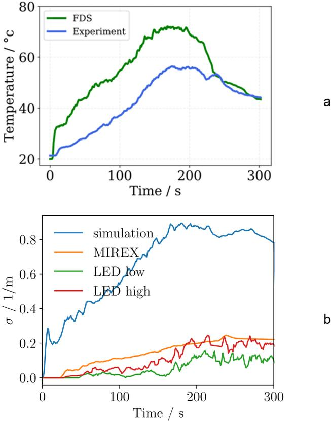
Fig. 5. Simulation results for the temperature development (a) and light extinction coefficient (b) during the experiment.
