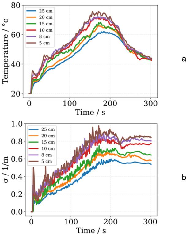
Fig. 3. Sensitivity of temperature (a) and extinction coefficient (b) w.r.t. the numerical grid resolution.
