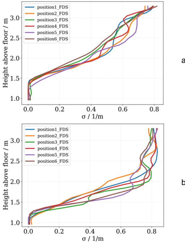
Fig. 4. Simulation results at  $t=150$  s (a) and  $t=250$  s (b) for the light extinction coefficient profiles at six selected positions in the compartment.
