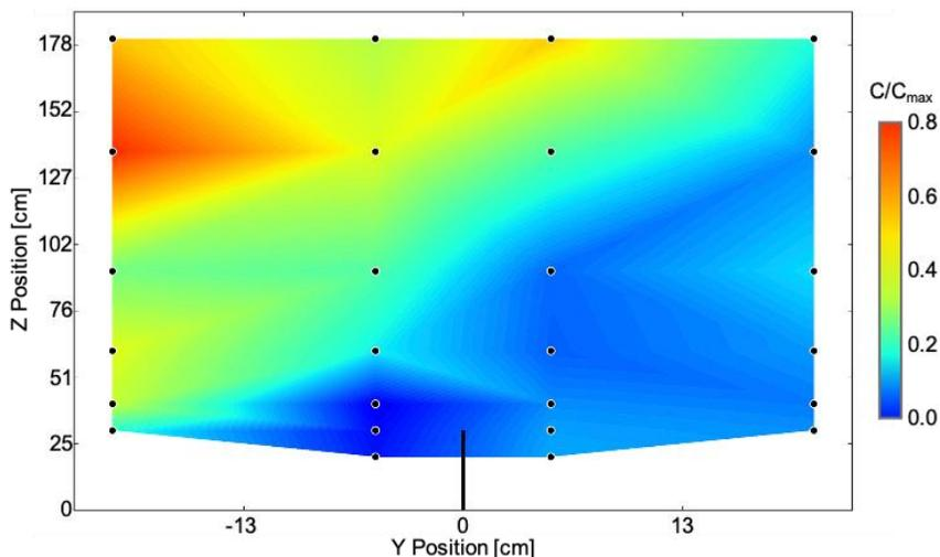
Fig. 3. Contour representation of relative methane concentrations.
