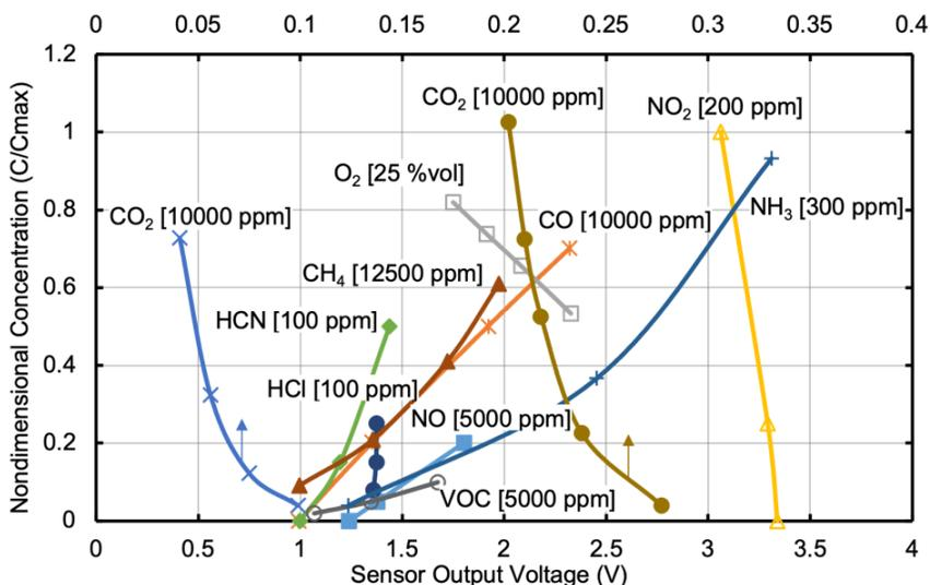
Fig. 2. Sample calibration set for sensor suite applied to testing.
