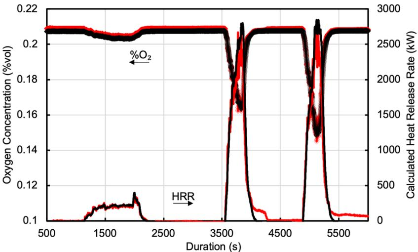
Fig. 5. Measured oxygen concentration and calculated heat release rate from traditional analyzers (red) and developed sensor suite (black).
