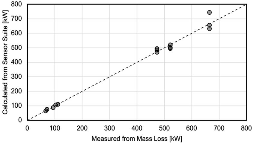
Fig. 4. Calibration of sensor suite heat release rate calculation.
