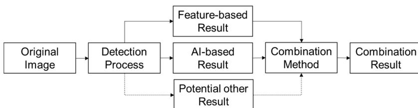
Fig. 1. Combination of the partial results of the different algorithms.
