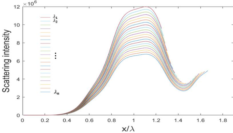
Fig. 2. Scattered light intensities of different particle sizes under irradiation of incident light with continuously varying wavelengths. The curves of different colors represent the continuously changing wavelength of the incident light, and the wavelength of the incident light corresponding to the curve increases from bottom to top. The range of particle sizes on each curve is the same.
