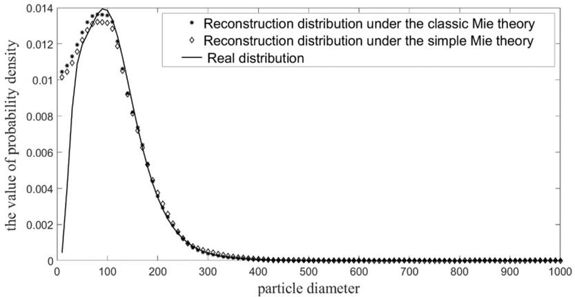
Fig.3. A particle spectrum that satisfies a bimodal log-normal distribution with median values of 70 nm and 130 nm and standard deviations of 1.75 and 1.45, and its reconstruction results under our method.
