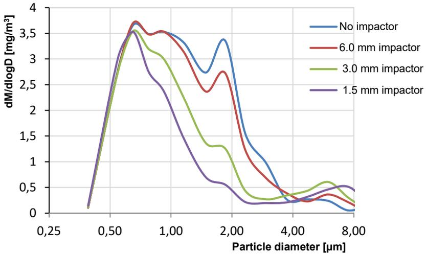
Fig. 5. Mass distribution of aerosol with different impactors.
