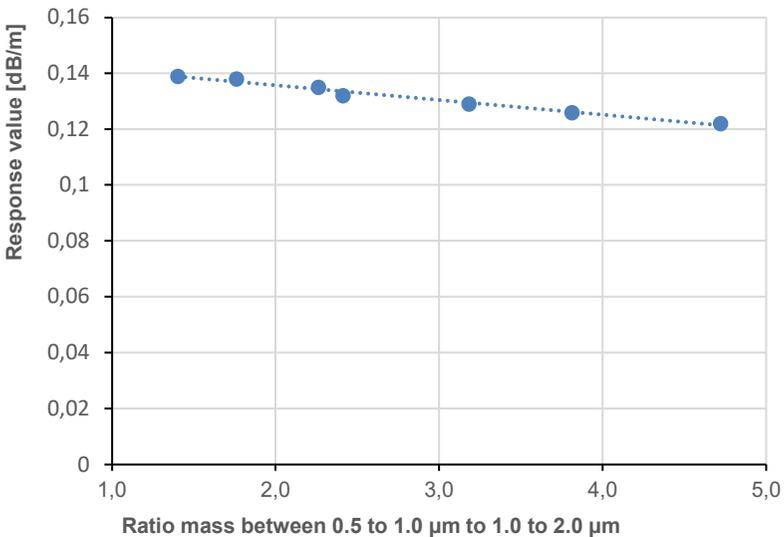
Fig. 7. Effect aerosol mass distribution on detector response value.
