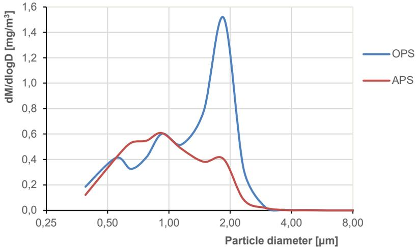
Fig. 3. Mass distribution of aerosol in Lorenz test tunnel with AGW aerosol generator.
