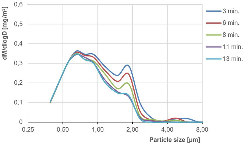
Fig. 6. Mass distribution of aerosol after aging in tunnel.
