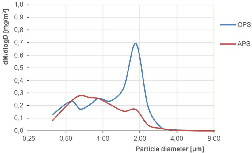
Fig. 2. Mass distribution of aerosol in AW Technology 2800 smoke/heat detector test tunnel.
