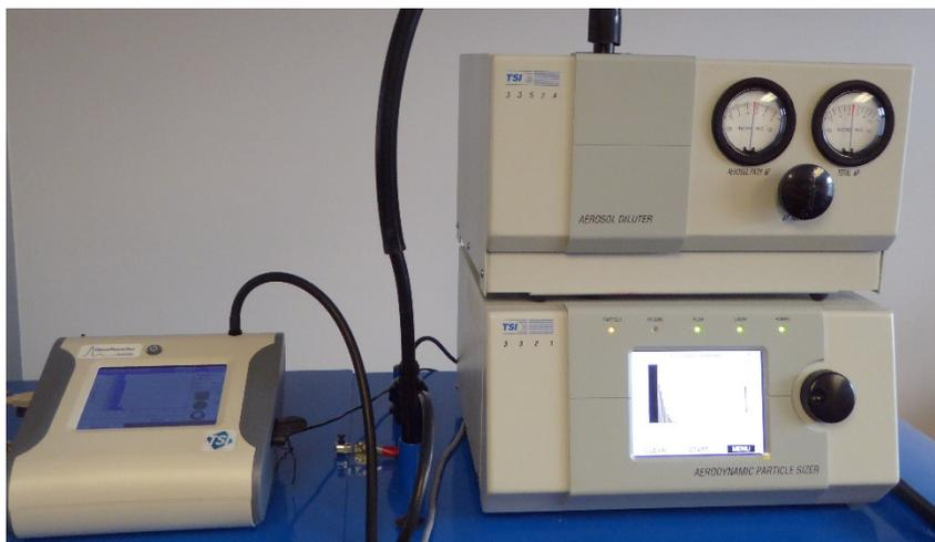
Fig. 1. TSI 3330 OPS instrument (left) and TSI 3321 APS instrument (right) with diluter on top of detector test tunnel.
