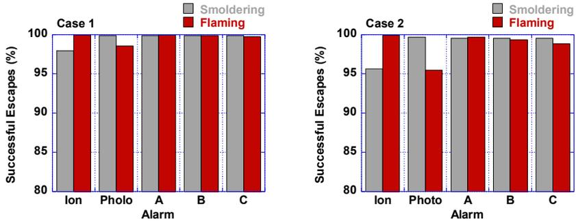
Fig. 1. Case 1) Smoke alarm in RFO and occupant in the RFO or any other room. Case 2) Smoke alarm and occupants located outside the RFO.
