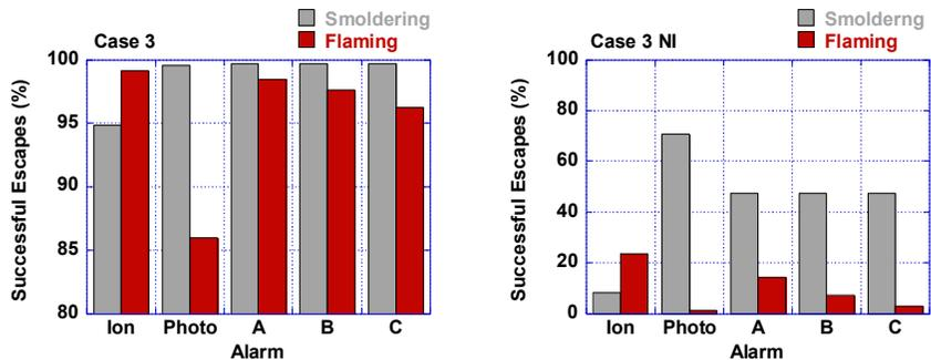
Fig. 2. Case 3) Smoke Alarm and occupant needing rescue located in RFO. Case 3 NI) Case 3 configuration without smoke alarm interconnection.
