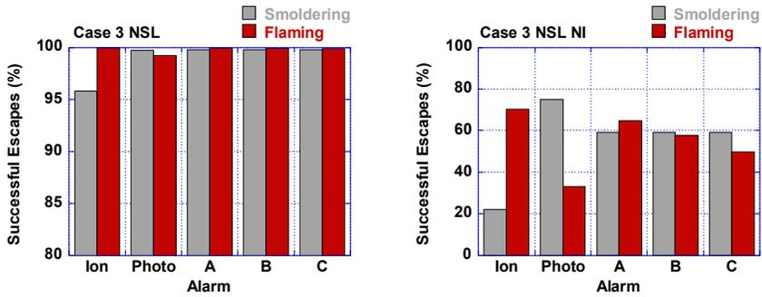
Fig. 3. Case 3 NSL) Smoke Alarm and occupant needing rescue located in RFO with smoke limit not enforced. Case 3 NSL NI) Case 3 configuration with smoke limit not enforced and without smoke alarm interconnection.
