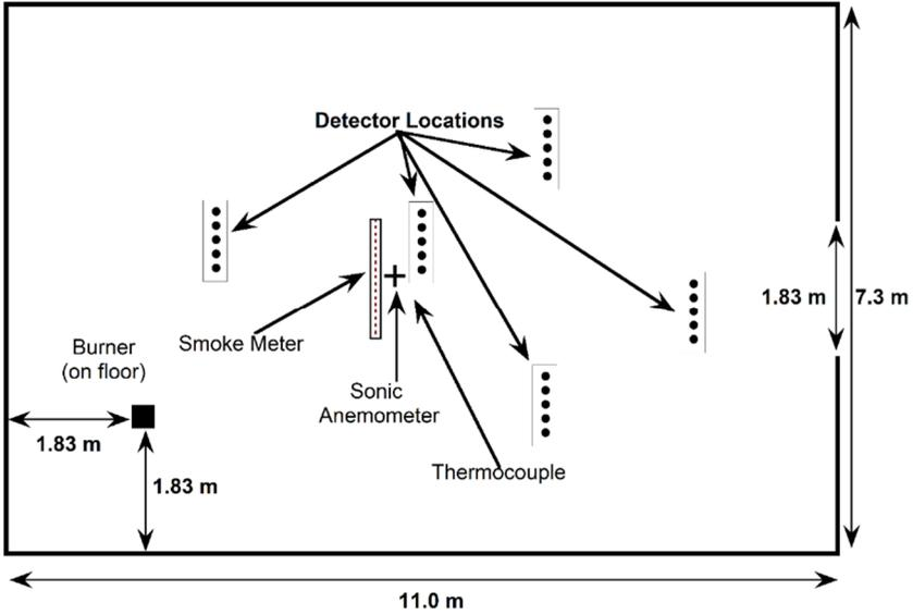
Fig. 1. Schematic diagram showing the placement of ceiling-mounted detectors (small circles), a ceiling smoke meter and the burner fire source (floor location) for the smooth ceiling configuration.
