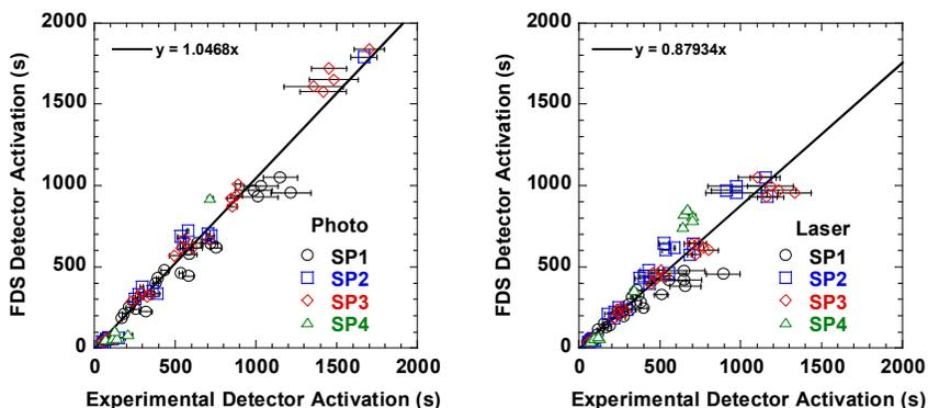
Fig. 2. Beamed ceiling configuration predicted versus experimental detector activations for the photoelectric detector (left) and laser detector (right). The symbols represent the four different set points specified. The line and equation are for a linear best fit line passing through the origin. Error bars represent  $\pm$  one standard deviation of the repeated experimental values.
