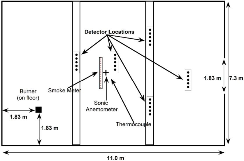
Fig. 2. Schematic diagram showing the placement of ceiling-mounted detectors (small circles), a ceiling smoke meter and the burner fire source (floor location) for the beamed ceiling configuration.
