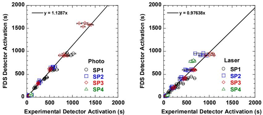
Fig. 1. Smooth ceiling configuration predicted versus experimental detector activations for the photoelectric detector (left) and laser detector (right). The symbols represent the four different set points specified. The line and equation are for a linear best fit line passing through the origin. Error bars represent  $\pm$  one standard deviation of the repeated experimental values.
