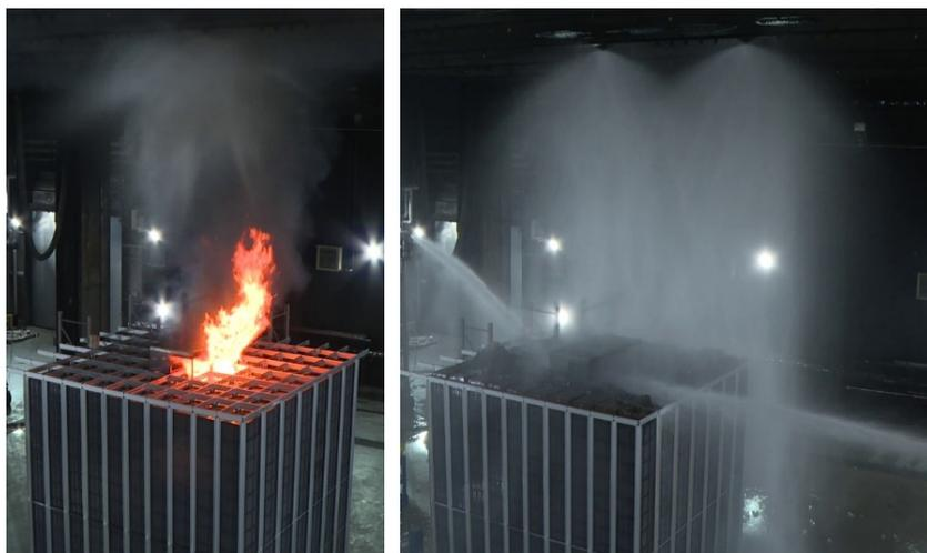
Fig. 1: Photos of Test 4 conducted with three robots located above the ignition area. The fire at first sprinkler operation shown on left and coupled operation of sprinklers and fire monitors shown on right.
