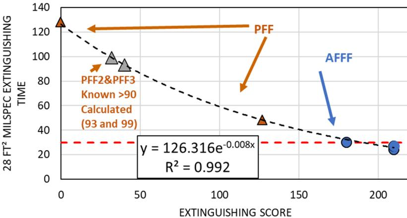
Fig. 7. Comparison between bench-scale extinguishing score and MIL-SPEC 28 ft<sup>2</sup> extinguishing time.
