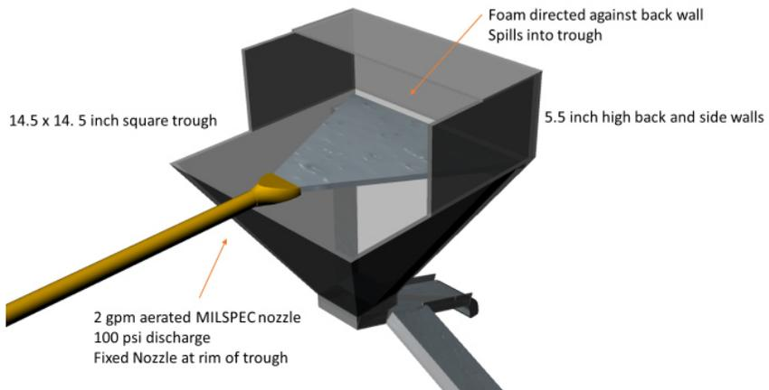
Fig. 2. Spray nozzle and foam collector and separator.
