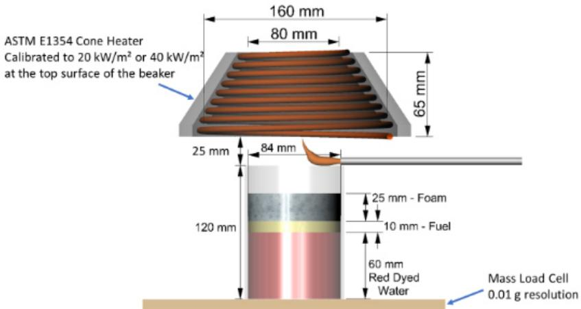
Fig. 5. Test configurations for stability of foam under external radiation.
