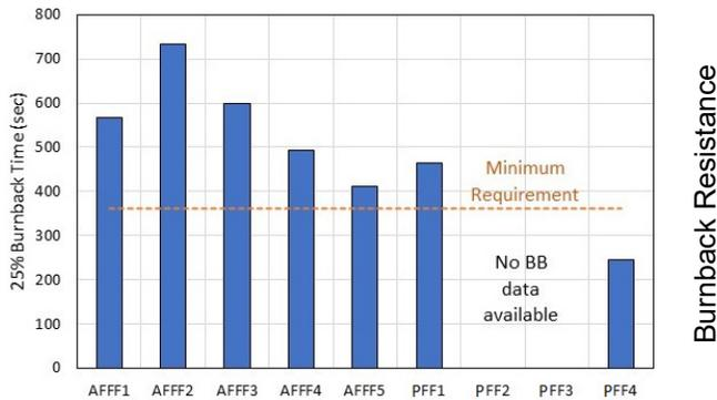
Fig. 1. MIL-SPEC scale results for evaluated foams.
