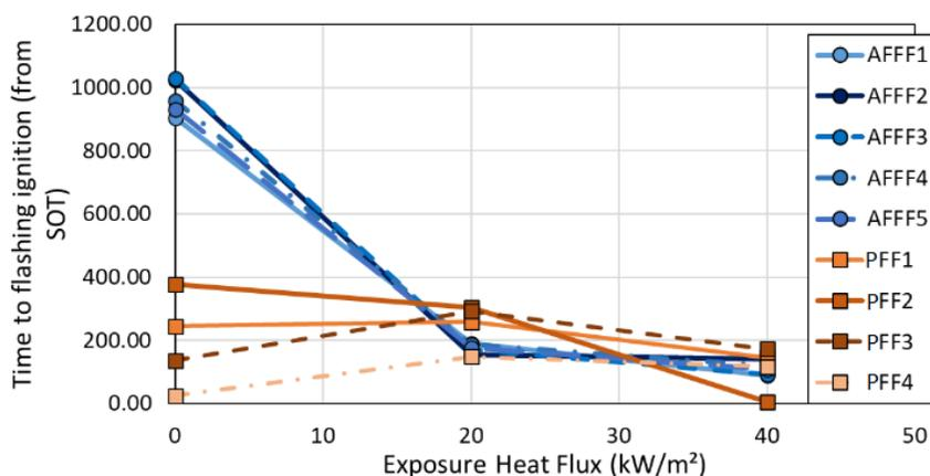
Fig. 6. Flash ignition times at different heat flux levels.
