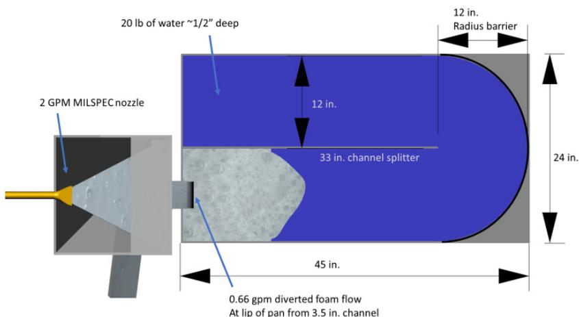
Fig. 3. Foam fluidity test pan and foam distributor.
