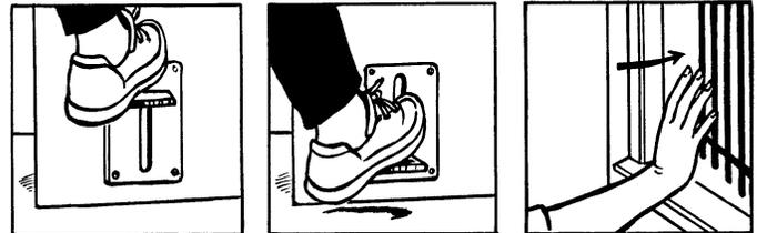
**Step down on pedal. Push open bars.**
