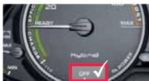
It may not be possible to detect that the car is ready to go by the noises it makes when in operation, as the electric motor is silent. If the large needle in the dial on the left of the instrument cluster (power metre) is not on „OFF“ (for example on the „READY“ position), you have to expect that the electric motor may run or the internal combustion engine may start automatically.
