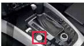
With the ignition switched on and the key **not** in the ignition (possible with the convenience key), the ignition can be switched off by pressing the start-stop button. If possible, take the convenience key outside the transmission range of the vehicle (1.5 m).
