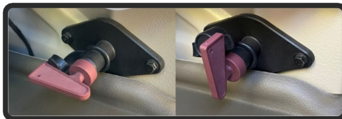
12V Switch ON
