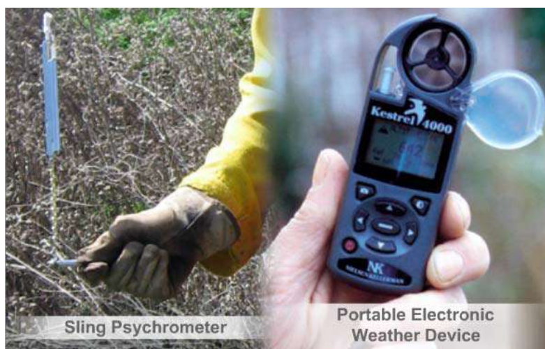
Caption: Examples of both a sling psychrometer (left) and a portable electronic weather device (right).
