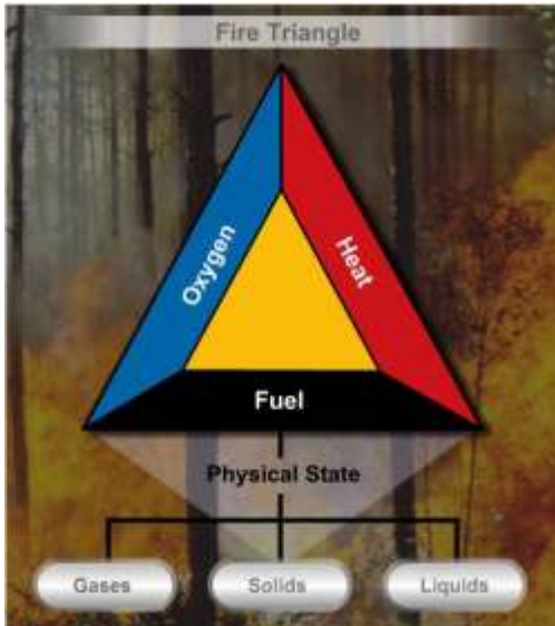
Caption: The fire triangle's sides represent the three components required for combustion—oxygen, heat, and a fuel source. These components can occur in three states including as a gas, a solid, or a liquid.
