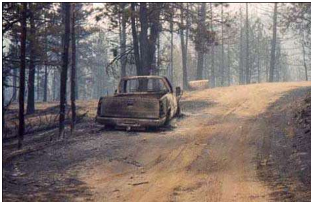
Caption: A severely fire-damaged truck from conducted heat from the exhaust system.
