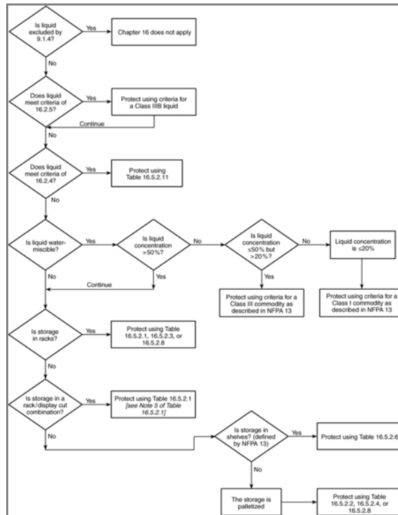
Figure 16.4.1(b) Fire Protection Criteria Decision Tree for Miscible and Nonmiscible Flammable and Combustible Liquids in Nonmetallic Containers.
