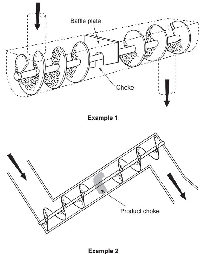
**Figure A-3-9.2(a) Screw conveyor chokes.**
