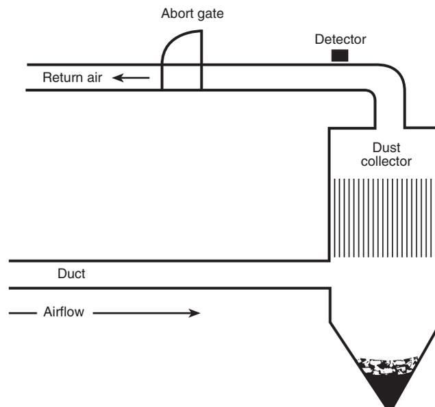
**Figure B-2.1** The minimum compliance spark detection system.
