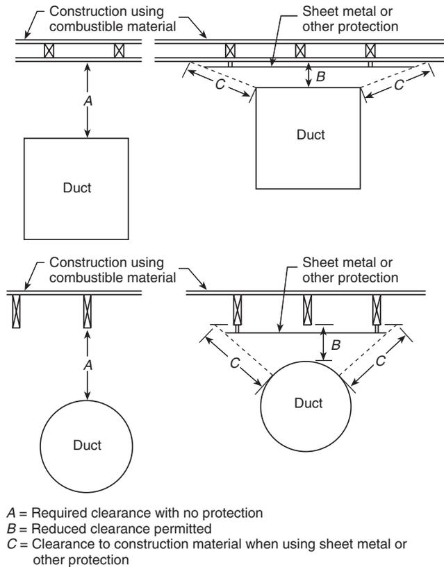
The protection applied to the construction using combustible material shall extend far enough in each direction to make C equal to A.
