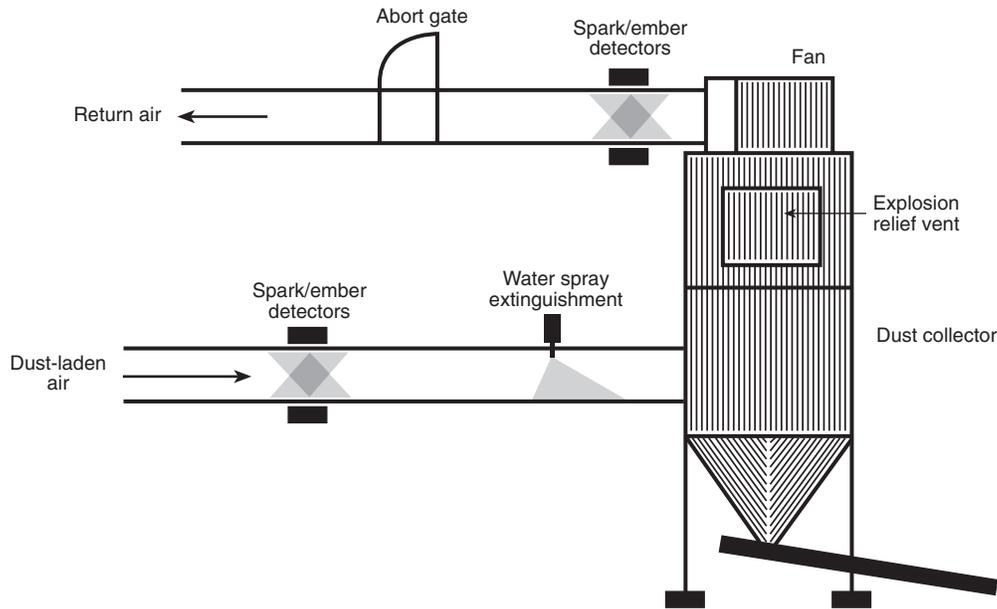
Figure B-2.4 The basic spark detection and extinguishment system for a single air-material separator.
