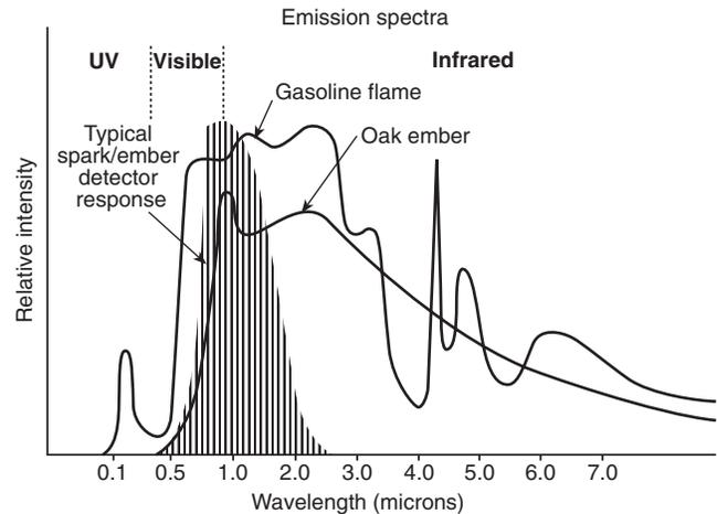
Figure B-1.6 The emissions of an oak ember and gasoline flame compared to the spectral sensitivity of a spark/ember detector.
