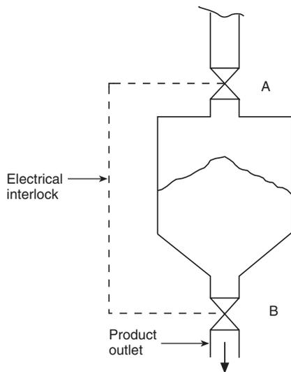
Note: Rotary valve A energized, B de-energized
