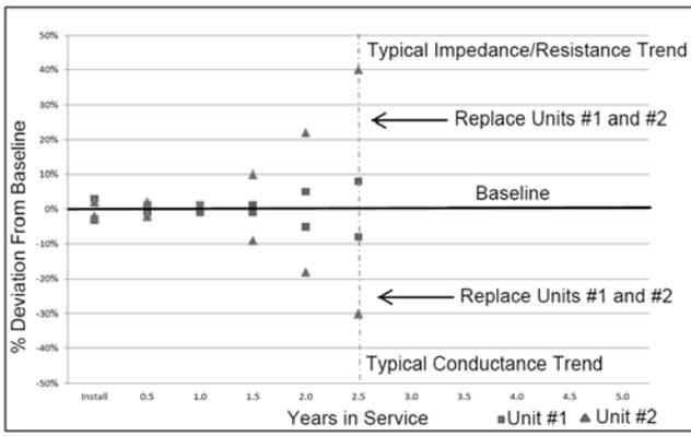
**FIGURE A.14.4.3.2 Item 9(d) Example Ohmic Trend Analysis for a 24 Volt Battery Made Up of Two 12 Volt Units.**
