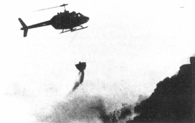
Figure A-5-2.3 (b) The use of helicopters has become a common occurrence in wildfire suppression. This helicopter is being used to make water drops on a wildfire.
