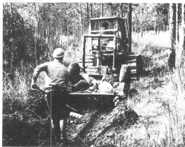
Figure A-5-2.2(b) Tractor plows are often used in suitable terrain to build firelines along the flanks and rear of a wildfire.
