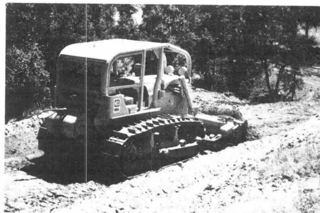
Figure A-5-2.2(a) Dozers are a valuable tool for wildfire suppression. This one is properly equipped with protective canopy, lights, brush guards, and a winch.
