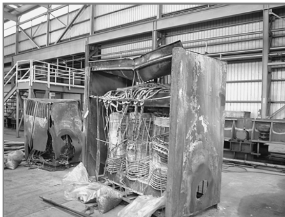
Figure L.7(b) Transformer (foreground) and Reactor Destroyed by Fault Current. (Courtesy of Shermco Industries, Inc.)
