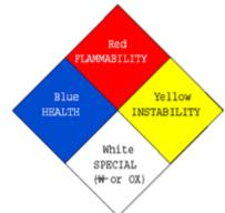
The six o'clock position on the symbol represents special hazards and has a white background. The special hazards in use are \(\psi\), which indicates unusual reactivity with water and is a caution about the use of water in either fire fighting or spill control response, and OX, which indicates that the material is an oxidizer.
