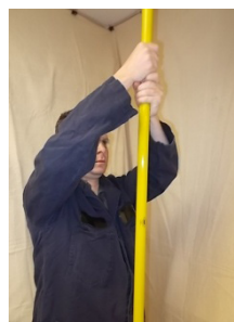
Figure 8.38.5.4 (a) Position of test subject body, arms, and hands with respect to pole. Photo Courtesy Intertek Testing Services. Used by Permission.
