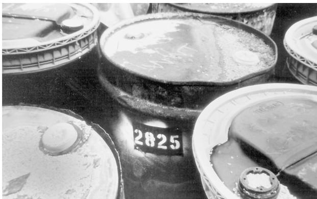
**EXHIBIT S6.2** Hazardous wastes can be found stored in containers, such as these barrels, that are corroded, lack appropriate identification labels, and are in poor condition.
