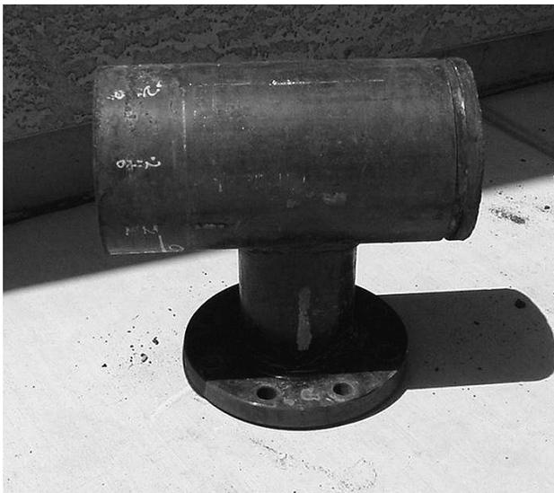
**EXHIBIT S3.2** Exterior View of Pipe with No Signs of Internal Corrosion.
